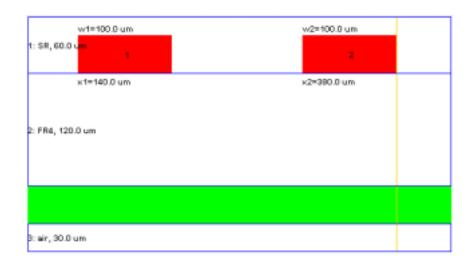
Figure 5.7: Coupled microstrips in a PCB layer.
