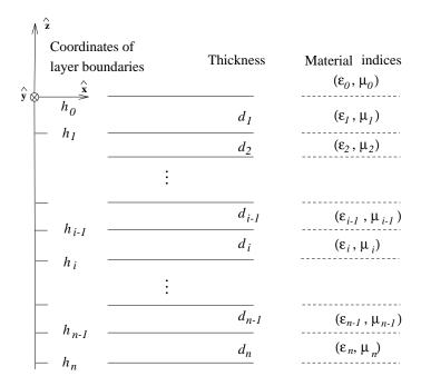
Figure 8.1: Description of dielectric layers with infinite lateral extent (in x, y directions). Either the top or the bottom side may be terminated by a perfect electric conductor (PEC).
