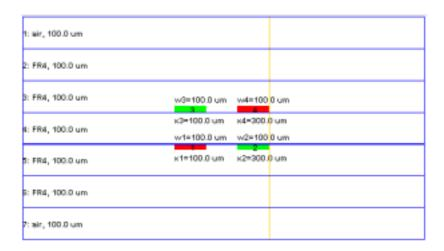
Figure 5.1: Broad-side coupled co-planar waveguide structure.
