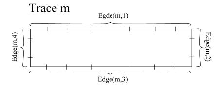
Figure 8.3: Edges of a typical trace are divided into line segments.
