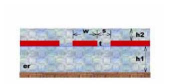
Figure 4.5: Bench mark case of ground backed coplanar waveguide with dielectric overlay.
