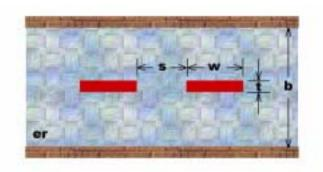
Figure 4.4: Bench mark case of two coupled striplines.
