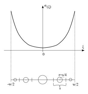
Figure 8.4: One typical edge of a trace.
