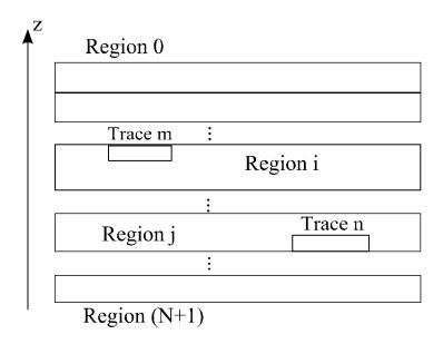
Figure 8.2: Traces in a multi-layered dielectric media.
