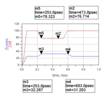
Figure 9.2: Time-domain verification of using RLGC data inside ADS.
