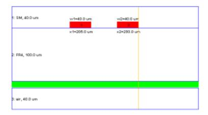
Figure 5.11: Coupled microstrips in a package layer.
