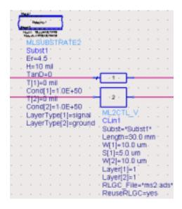
Figure 9.1: Using RLGC data inside an ADS design.
