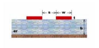
Figure 4.2: Bench mark case of two coupled microstrips.
