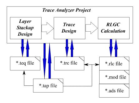
Figure 2.1: Typical work flow of using Trace Analyzer.
