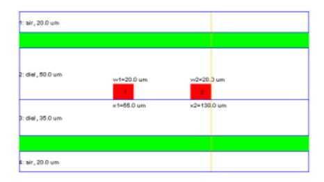
Figure 5.9: Coupled striplines in a package structure.
