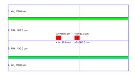
Figure 5.5: Coupled striplines in a PCB structure.
